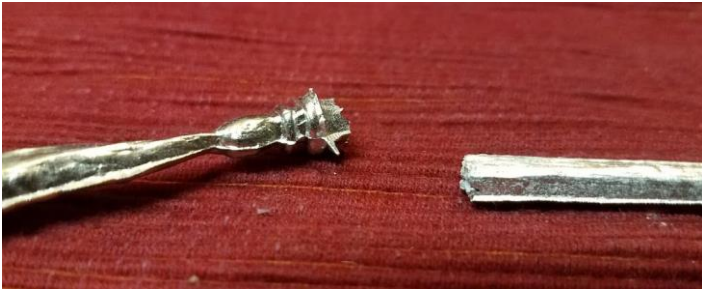
Figure C.8 – Simple knob with continuing weak spot issue.
