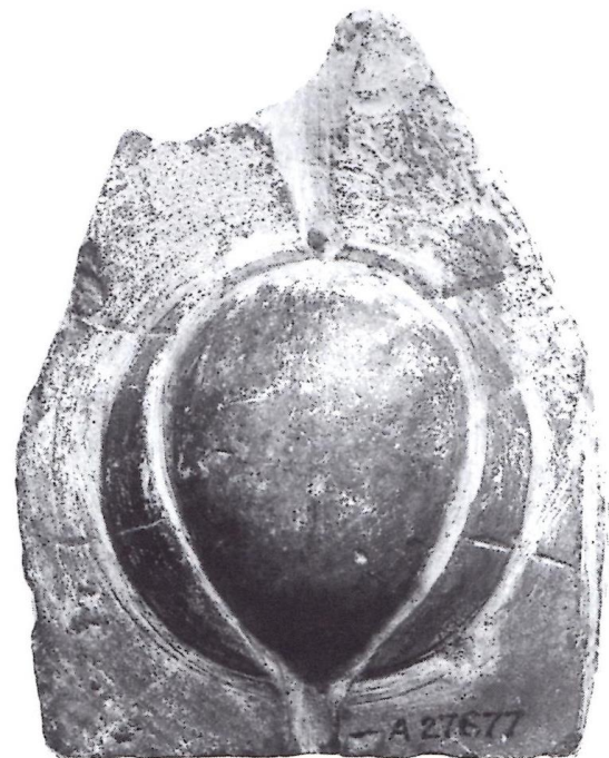
Figure 3 – c. 15 th century English fragment of a stone spoon mold. (Homer, 66)
