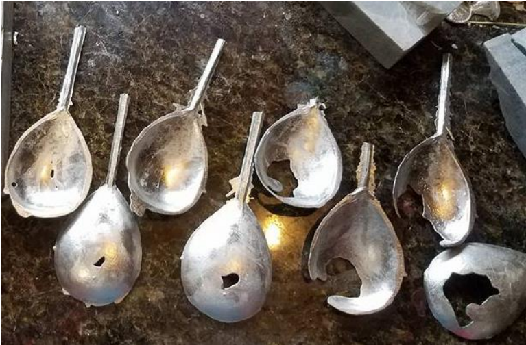
Figure C.5 – Progress of filling in bowl of spoon. These spoons would be quite effective “diet spoons”, allowing for little actual food to be eaten.
