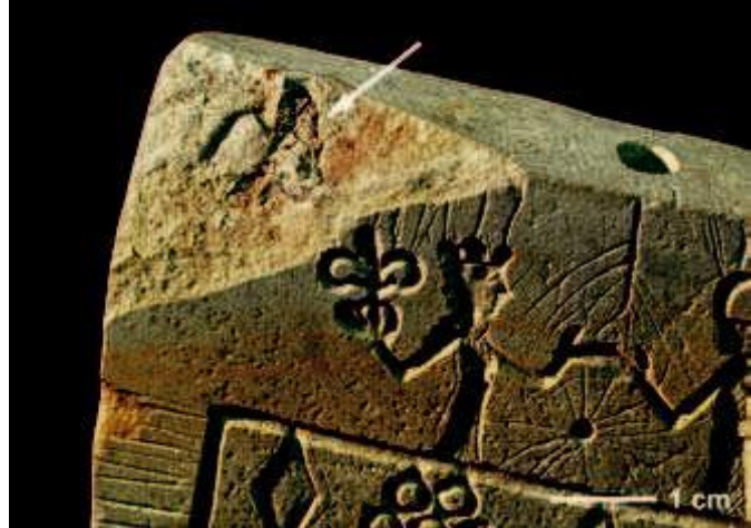
Figure 5 – Mold showing inner air vent hole that vents to larger side hole. Also show many air vent channels. Location: Magdeburg Date: before 1284 (Berger, 43)
