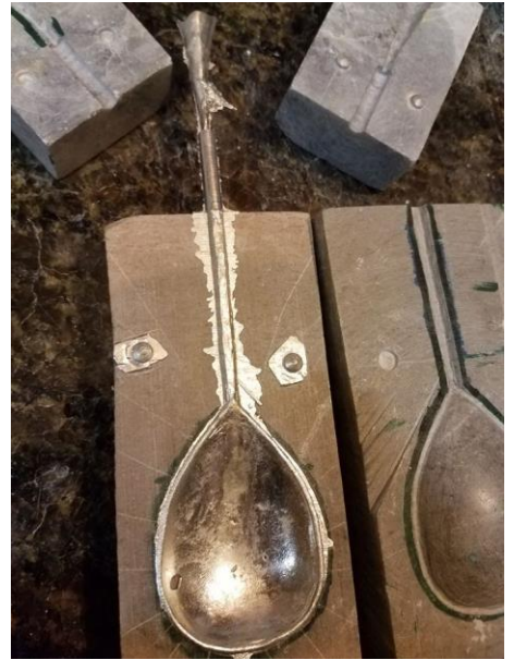
Figure C.6 – Spoon mold, including original throwaway knob
