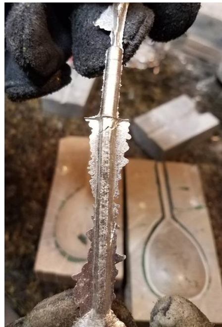
Figure C.4 – Example of weak spot near top of stem
