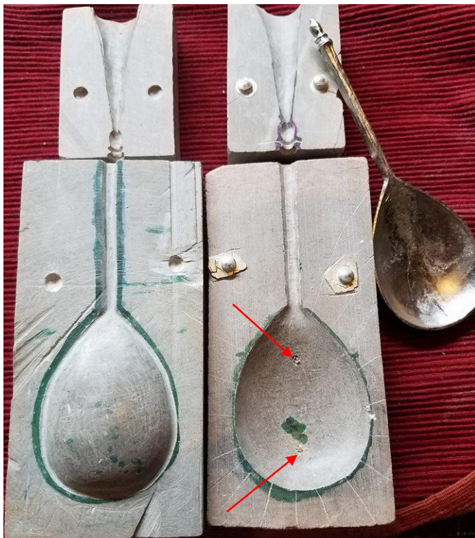
Figure C.7 – Spoon mold with simple knob mold top and completed spoon. Note two air venting holes in concave side.
