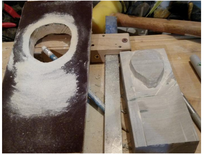
Figure C.2 – Sanding the base of the convex mold
