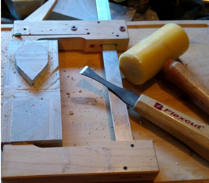
Figure C.1 – Roughing out the convex mold
