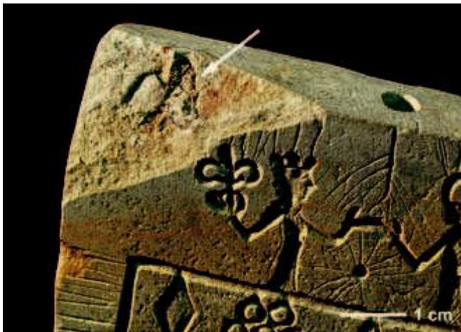
Figure 3 – Mold showing inner air vent hole that vents to larger side hole. Also show many air vent channels. Location: Magdeburg Date: before 1284 (Berger, 43)
